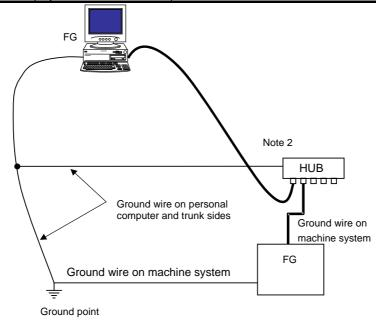
Wiring on a single ground point
