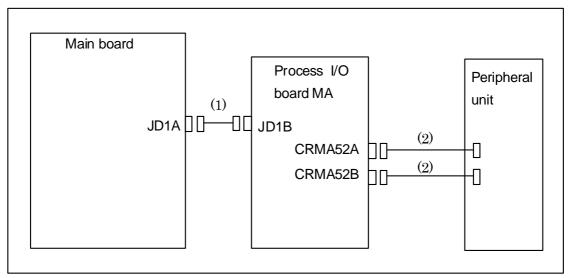
Fig.4.1.2 Block diagram of the process I/O MA
