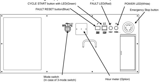
Fig.2.1 (i) R-30iB B-cabinet operator's panel
