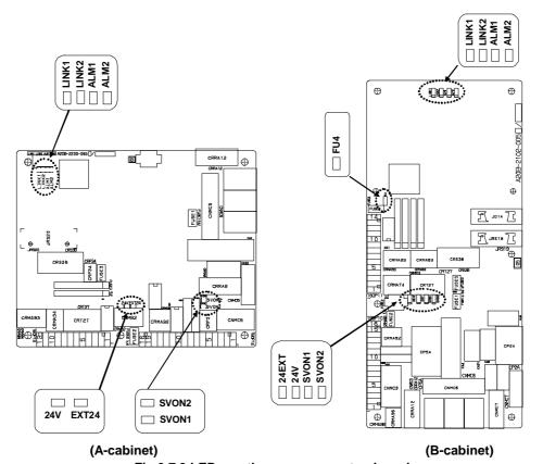
Fig.3.7.3 LEDs on the emergency stop board
