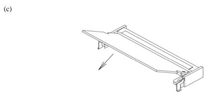
Fig.8.2 (g) Demounting/mounting a module
