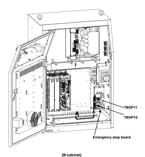
Fig.3.3.4 (a) Connection of the external power supply ON/OFF switch
