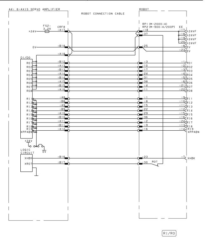
Fig.G.7(q) RI/RO connection diagram (Group 9:M-900iA/200P)
