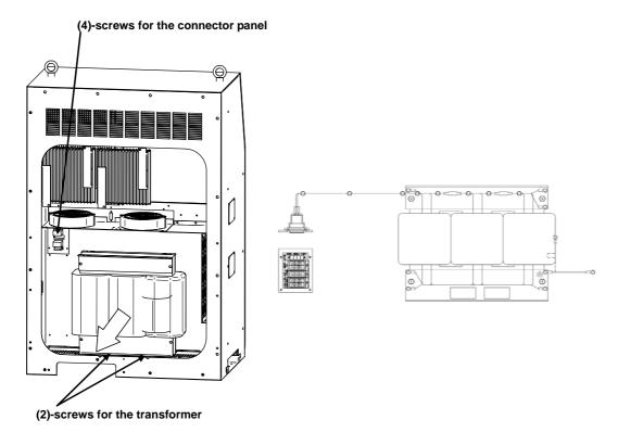
(4) Install a replacement transformer by reversing above steps.
