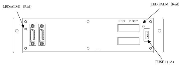
Fig.3.6 (e) Fuse on the process I/O board MA
