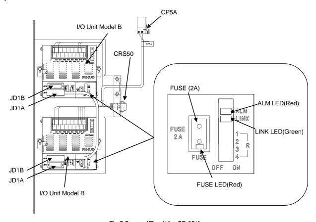
Fig.7 Sensor I/F unit for CR-35iA
