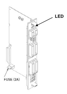
Fig.3.7.4 (a) LEDs on the Process I/O board JA/JB
