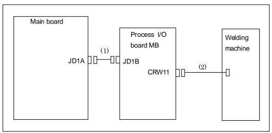
Fig.4.1.3 Block diagram of the process I/O MB
