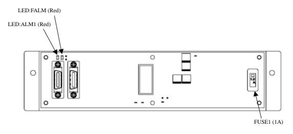
Fig.3.6 (f) Fuse on the process I/O board MB
