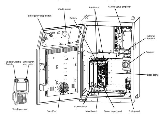
Fig.2.1 (e) R-30iB B-cabinet interior (Front)
