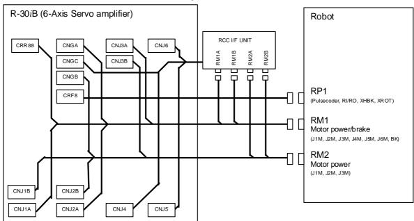
Fig.3.3.1 (c) Robot connection cable (Group4)
