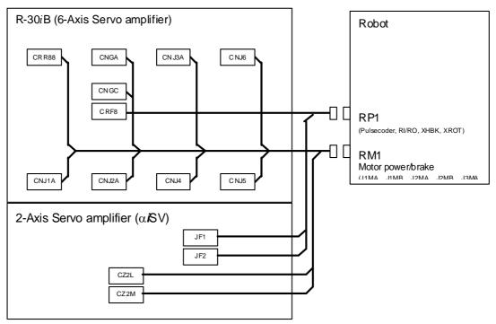
Fig.3.3.1 (e) Robot connection cable (Group6)
