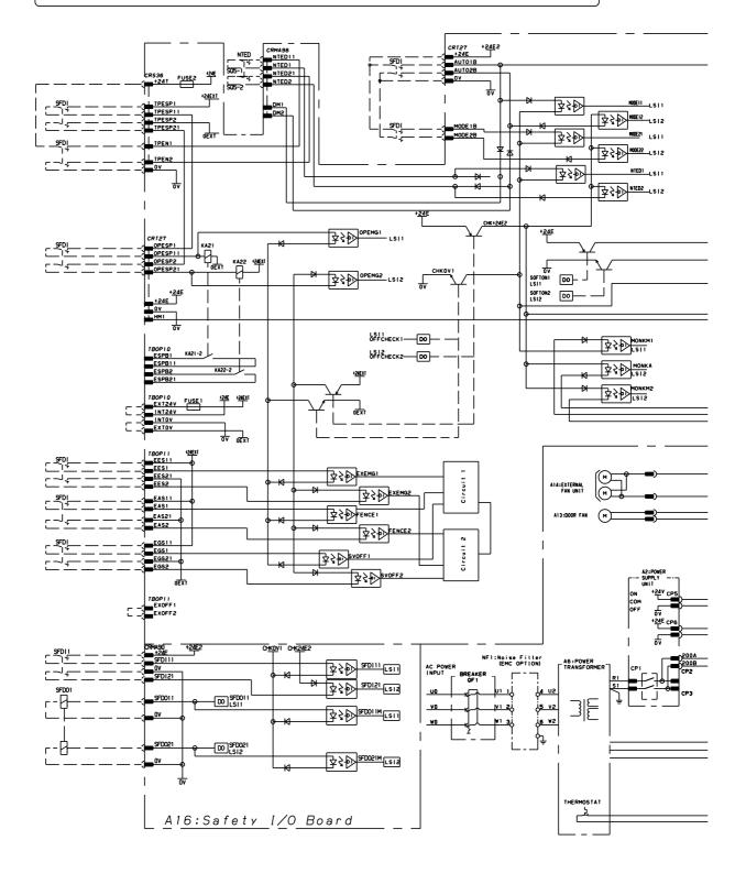
Fig.G.7(I) Emergency circuit connection diagram (B-cabinet/Power supply regeneration/Controller 2)
