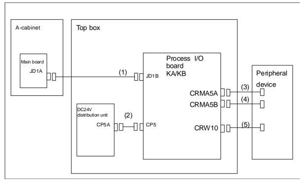
Fig.4.1.4 Block diagram of the process I/O board KA/KB
