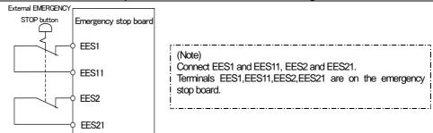
Fig. 3.1 Connection Diagram for External Emergency Stop Button
