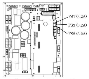
Fig.3.6(b) Fuse on the Servo amplifier
