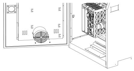
(Replacing the Door Fan Unit)
