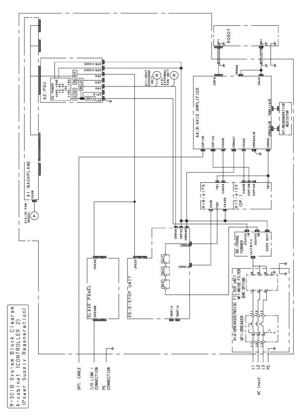
Fig.G.7(b) System block diagram (A-cabinet/Power supply regeneration/Controller 2)
