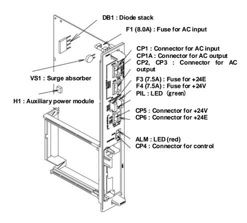
Fig.6.3 Interface of the power supply unit
