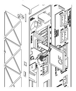
2. Lock the latch, and drive the screw.
