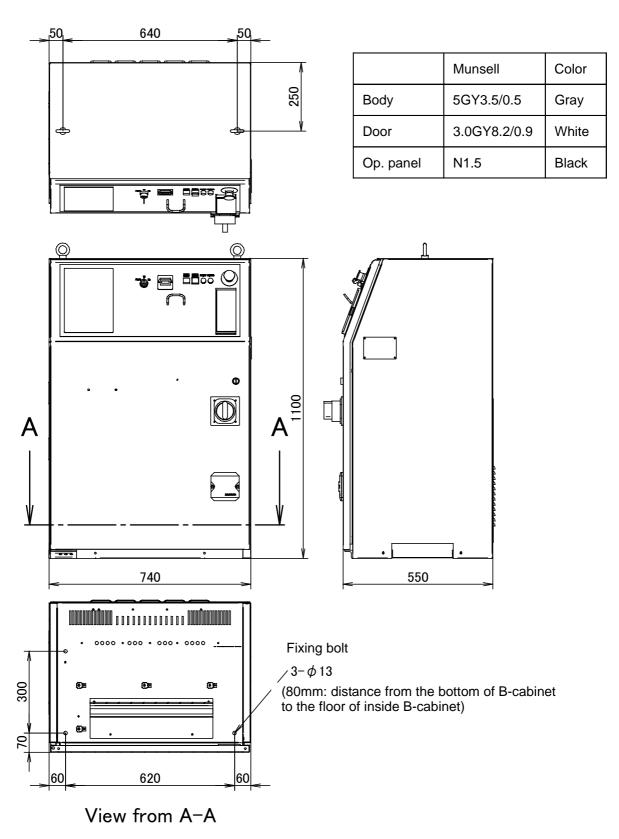
Fig.5.2.1(b) External dimensions (B-cabinet)
