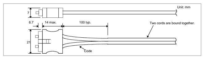
Fig.D (c) External dimensions of internal optical cable Unit: mm
