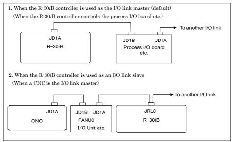
Fig.3.2.1 Connection of I/O links
