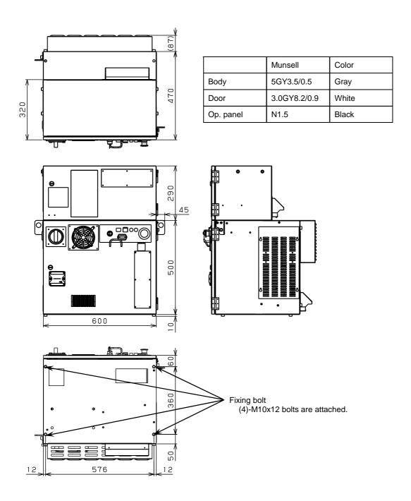
Fig.5.2.1(a2) External dimensions (A-cabinet with Top box)
