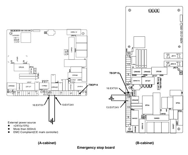
The relays for emergency stop input and output can be separated from controller's power. Please connect external +24V instead of internal +24V, if emergency stop output must not be effected controller's power.
