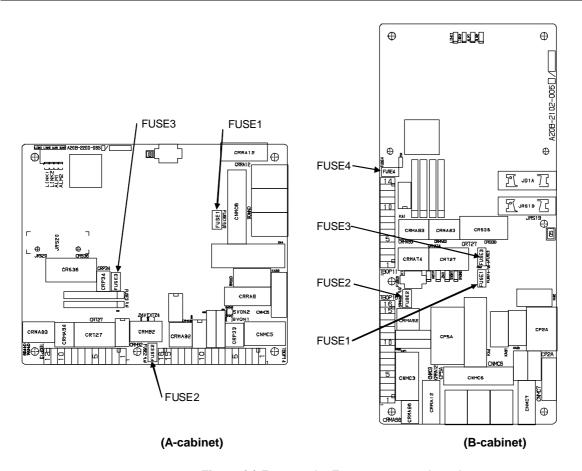
Fig.3.6 (c) Fuse on the Emergency stop board
