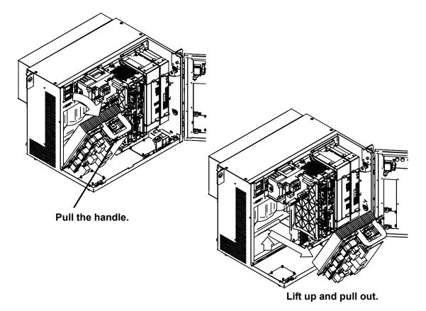
Fig.8.7(a) Replacing the servo amplifier (A-cabinet)
