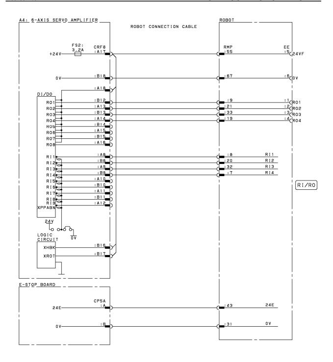
Fig.B (ad) RI/RO Connection Diagram (Group7; M-430iA/2P)
