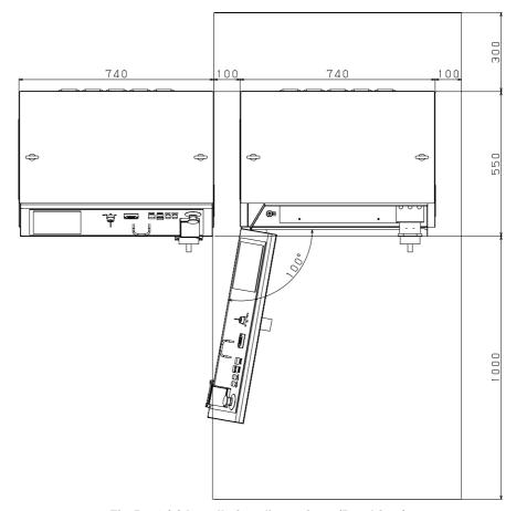
Fig.5.2.1 (e) Installation dimensions (B-cabinet)
