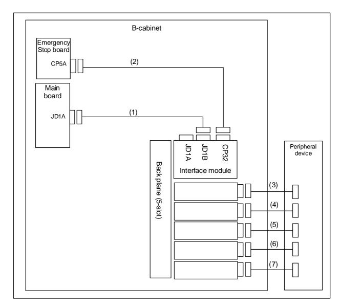
Fig.4.1.5.2 Block diagram of I/O Unit-MODEL A (In case of B-cabinet)
