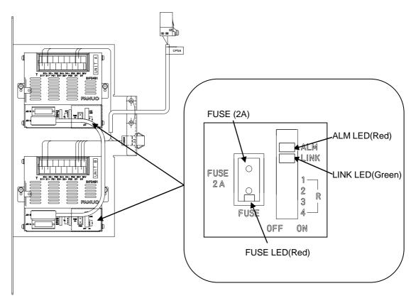
Fig.3.7.7 LEDs on the sensor I/F unit for CR-35iA
