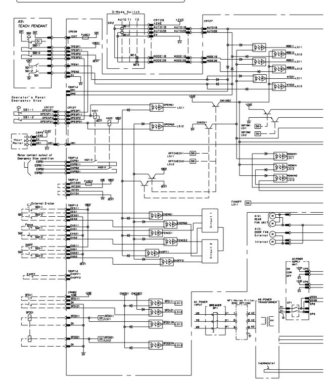
Fig.B (j) Emergency stop circuit connection diagram (A-cabinet/Power supply regeneration)
