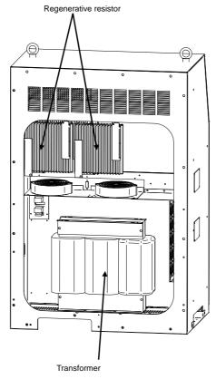
Fig.2.1 (g) R-30iB B-cabinet interior (Rear)
