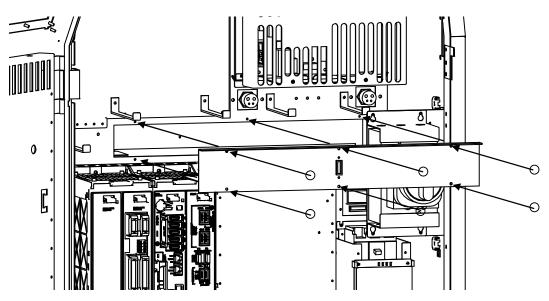
(Replacing the External Fan Unit)
