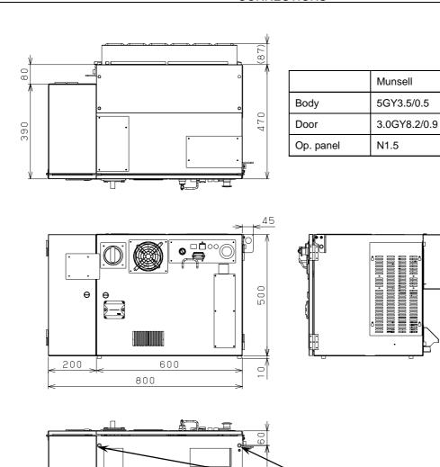
Fig.5.2.1(a3) External dimensions (A-cabinet with Side box)
