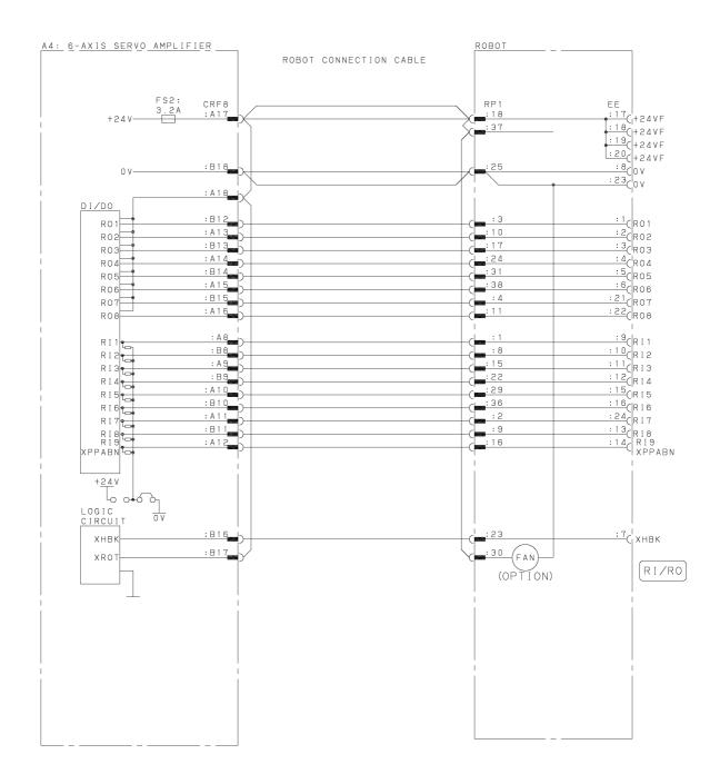
Fig.B (af) RI/RO Connection Diagram (Group11; M-2iA,M-3iA)
