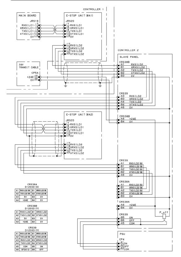
Fig.G.7(m) Connection between controller 1 and 2 (A-cabinet)
