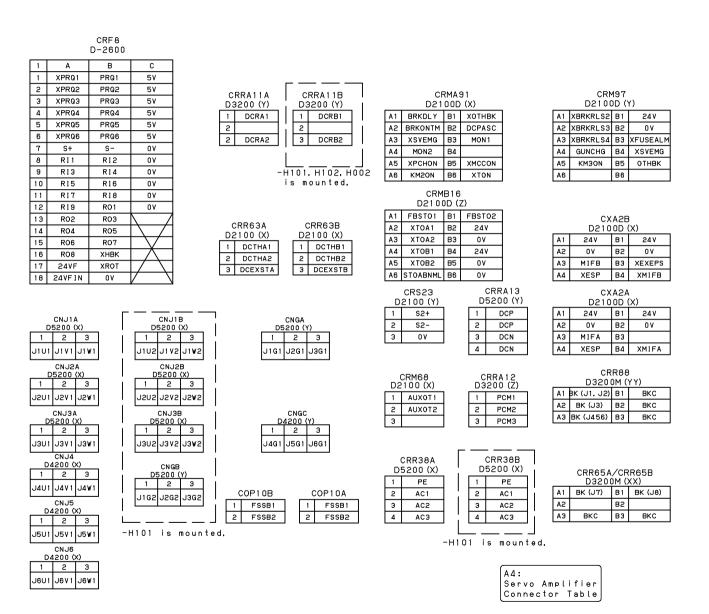
Fig.B (r) Servo amplifier connector table
