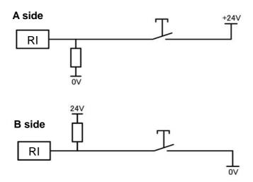
Fig.5.2 Circuit based on jumper pin location or setting of switch
