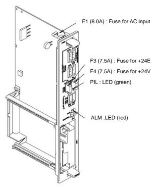
Fig.3.7.2 LEDs on the power supply unit
