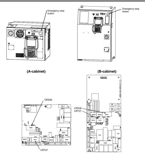
(Emergency stop board/A-cabinet) (Emergency stop board/B-cabinet) Fig.3.5 (a) SRVO-001 Operator panel E-stop
