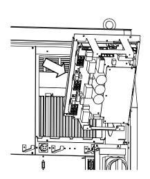
Fig.8.7(b) Replacing the servo amplifier (B-cabinet)
