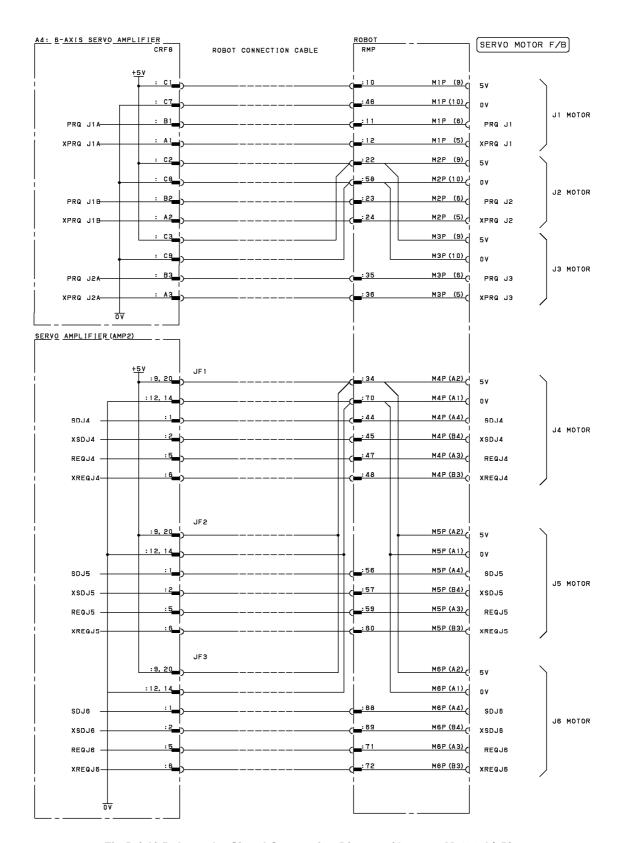
Fig.B (ak) Pulsecoder Signal Connection Diagram (Group7; M-430iA/2P)
