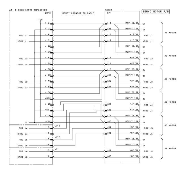
Fig.B (ah) Pulsecoder Signal Connection Diagram (Group5; M-900iA/400L,600,M-900iB/400L,700)
