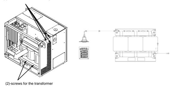
(6) Install a replacement transformer by reversing above steps.
