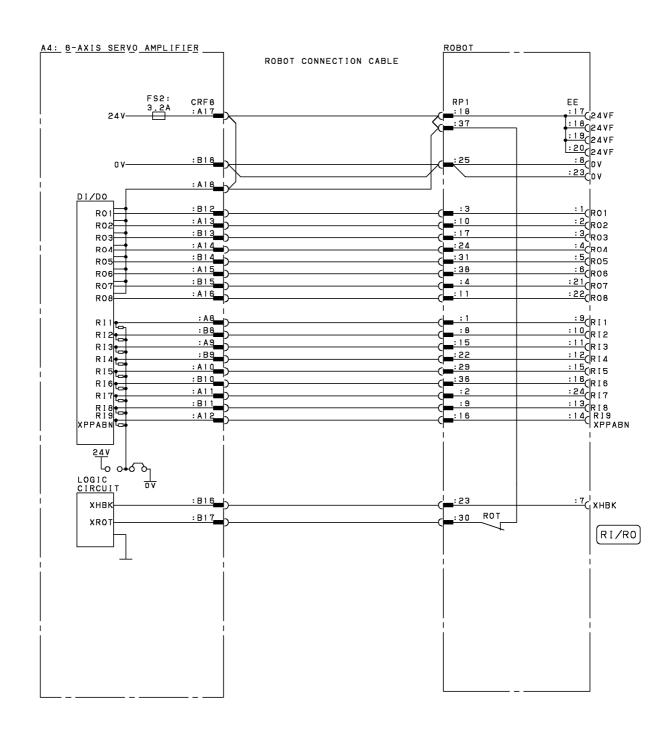
Fig.B (ab) RI/RO connection diagram (Group1 to 5)
