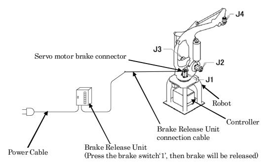
Fig.E.3.1 (c) How to connect brake release unit (In case of M-410iB)
