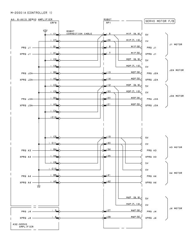
Fig.G.7(w) Pulsecoder signal connection diagram (Group 10:M-2000iA, Controller 1)
