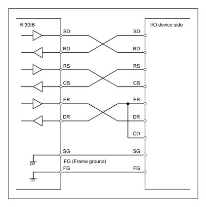
• The figure below shows a connection without the handshaking of the RS/CS, ER/DR signals.
