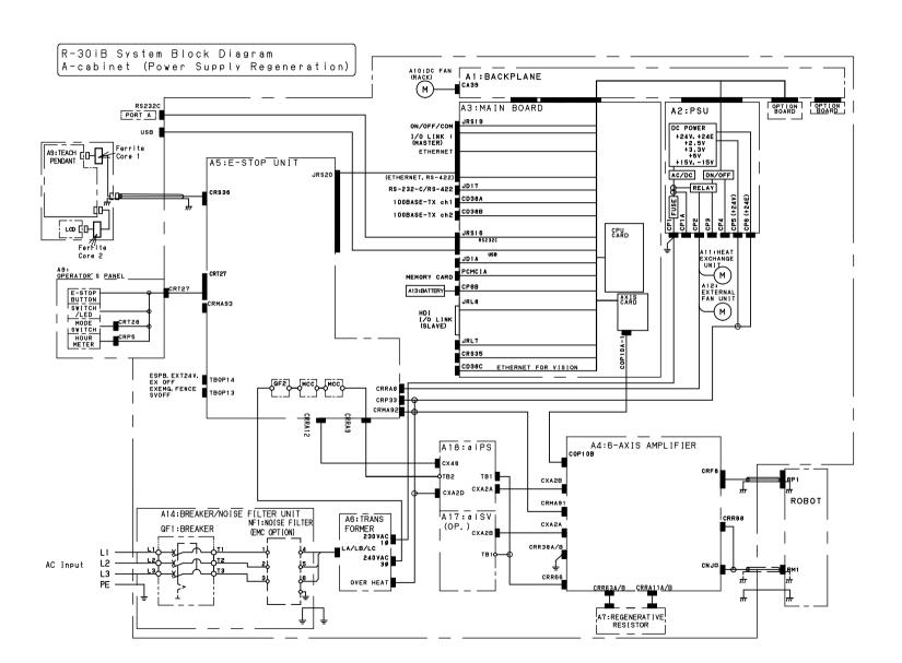
Fig.B (b) System block diagram (A-cabinet / Power supply regeneration)
