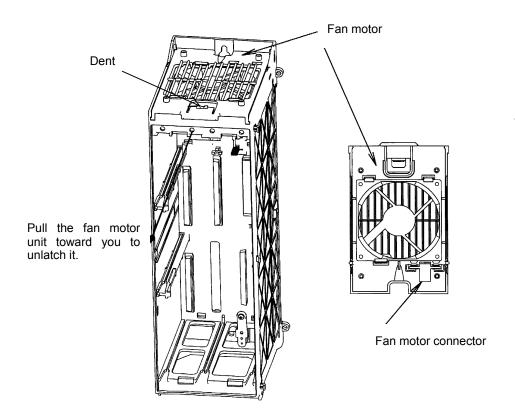
Fig.8.10 Replacing the control section fan motor
