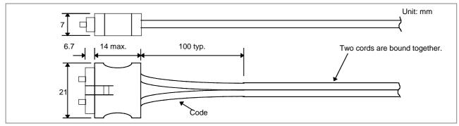
Fig.D (b) External dimensions of external optical cable Unit: mm
