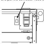
Fig.8.11.2 Replacing rear fan unit (A-cabinet)
