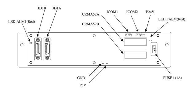
Fig.4.6 Process I/O board MA
