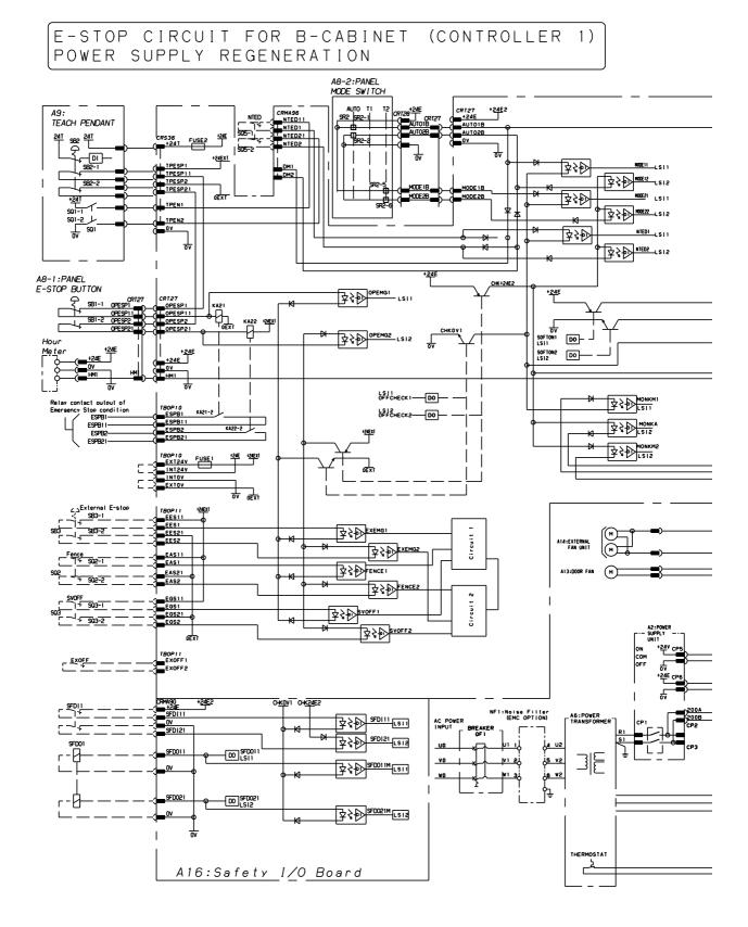
Fig.G.7(k) Emergency circuit connection diagram (B-cabinet/Power supply regeneration/Controller 1)
