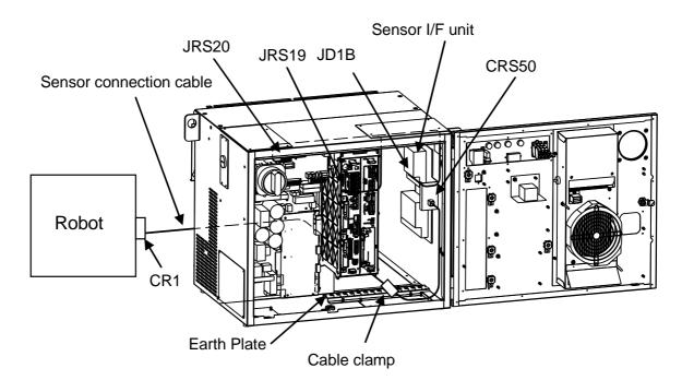
Fig. 4.11 Connecting the sensor connection cable
