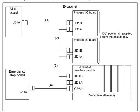
Fig.4.1.6.1 Block diagram of two or more process I/O printed circuit boards and I/O unit-MODEL A (In case of B-cabinet)
