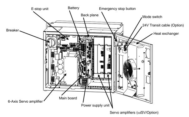
Fig.2.1 (b) R-30iB A-cabinet interior (Front)
