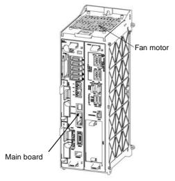
Fig.3.5 (s) SRVO-123 Fan motor rev slow down(%d)
