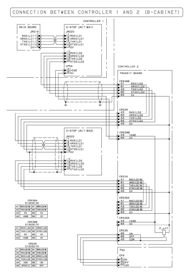
Fig.G.7(n) Connection between controller 1 and 2 (B-cabinet)
