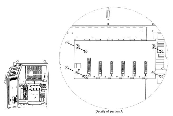
Fig.8.8.1 Replacing the base unit of I/O unit model A
