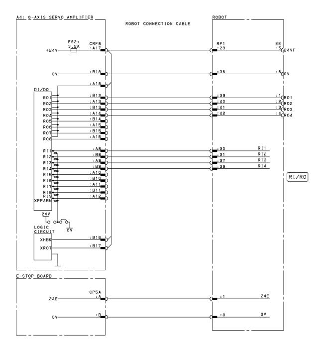
Fig.B (ac) RI/RO Connection Diagram (Group6; M-430iA/2PH,4FH)
