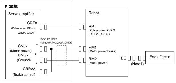
Fig.3.1 (a) Mechanical connection diagram
