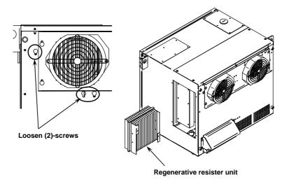
(4) Remove four screws at the code grip panel and pull out the cable together with the panel. Then the regenerative resister unit is separated from A-cabinet.
