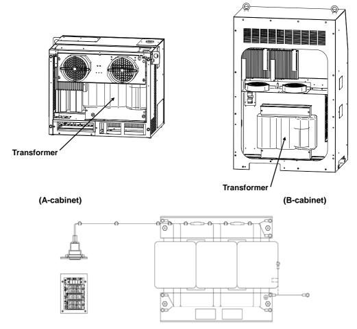
Fig.6.2 (a) Transformer mounting locations and structure
