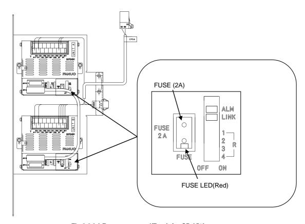
Fig.3.6 (g) Fuse on sensor I/F unit for CR-35iA
