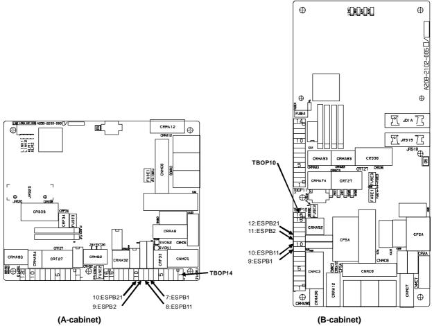
Fig. 3.3.5 (b) Emergency stop board
