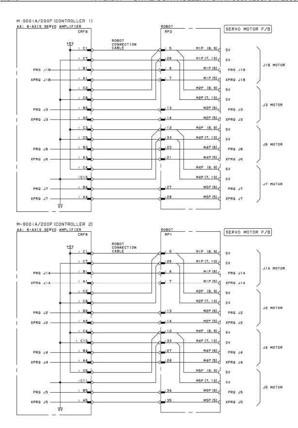
Fig.G.7(r) Pulsecoder signal connection diagram (Group 9:M-900iA/200P)
