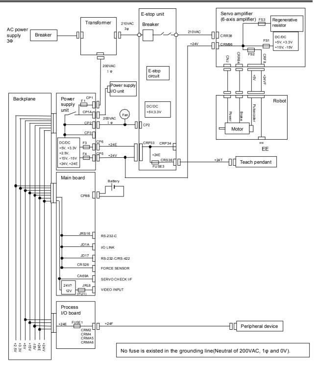
Fig.6.1 Block diagram of the power supply
