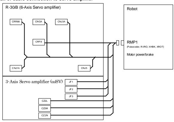
Fig.3.3.1 (f) Robot connection cable (Group7)
