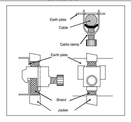
For protection against the noise, cut part of the jacket of the connection cable to expose the shield, and fasten this part to the earth plate with the cable clamp.
