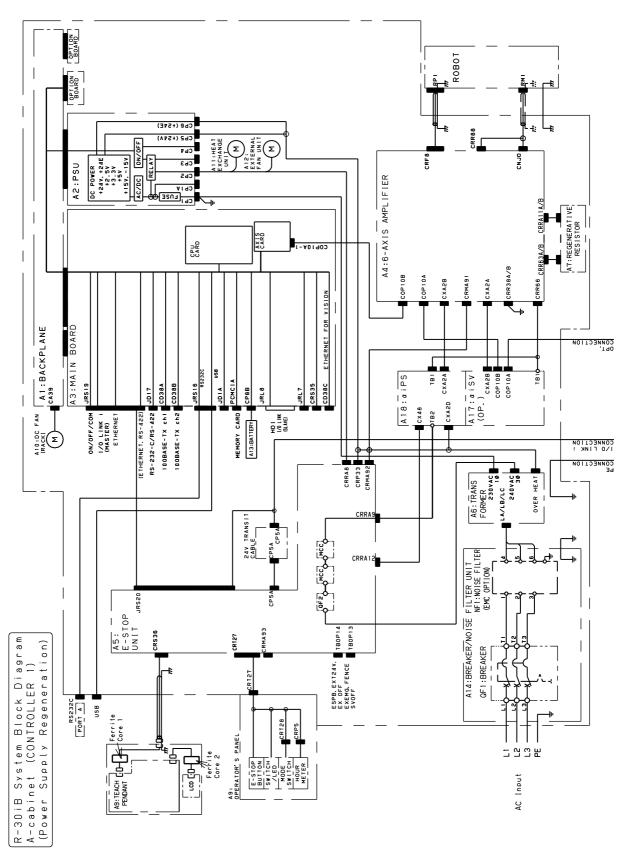
Fig.G.7(a) System block diagram (A-cabinet/Power supply regeneration/Controller 1)
