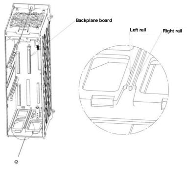
Fig.8.1.2 (a) Replacing the backplane board
