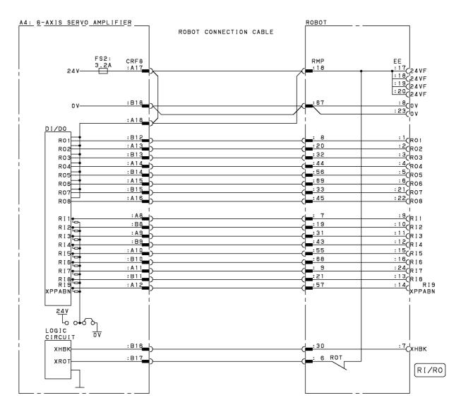
Fig.B (ae) RI/RO Connection Diagram (Group8; ARC Mate 100iC, ARC Mate 120iC)
