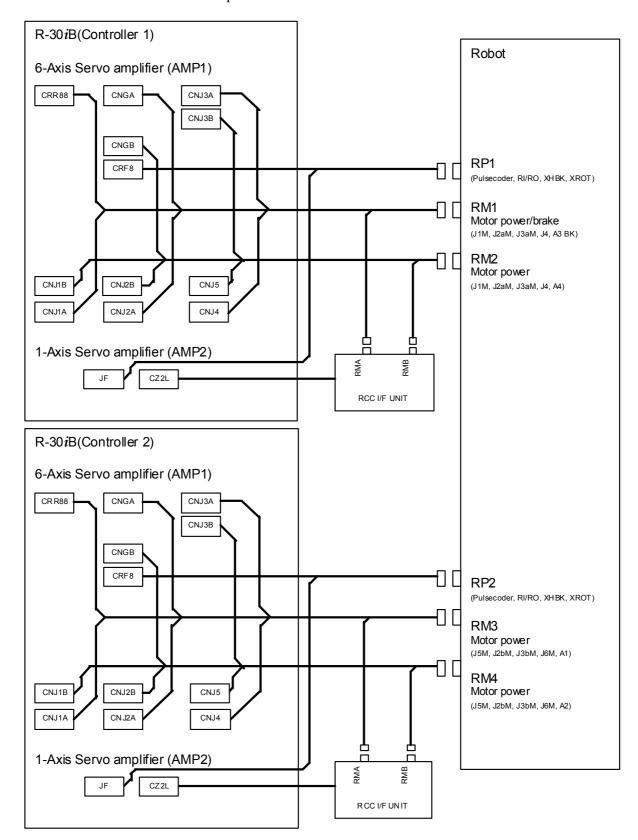
Fig.G.4(b) Robot connection cable (Group10: M-2000iA)
