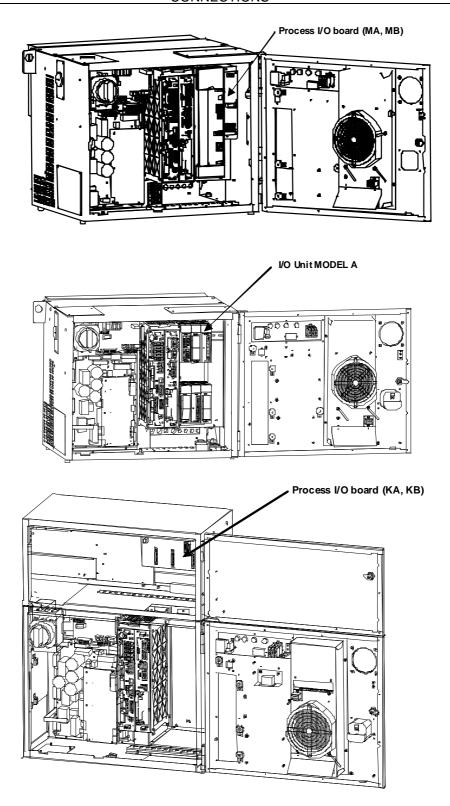
Fig.4(a) Locations of peripheral device interfaces (A-cabinet)
