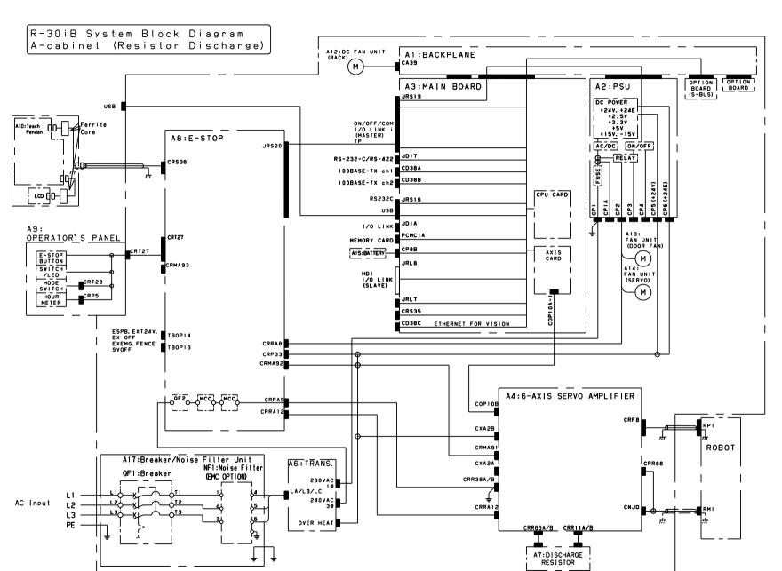
Fig.B (a) System block diagram (A-cabinet / Resistor discharge)
