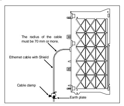
The Ethernet cable must be fastened by a cable clamp to prevent tension being applied to the modular connector (RJ-45) that connects the cable to the controller even if the Ethernet cable is pulled directly. This clamp is also used to ground the cable shield.
