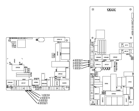
(Emergency stop board/A-cabinet) (Emergency stop board/B-cabinet) Fig.3.5 (e) SRVO-007 External E-stop
