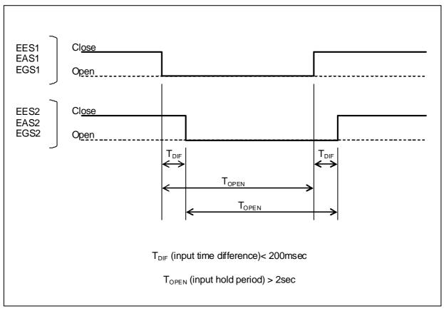
Fig.3.3.5(c) Input timing of duplicate safety signals
