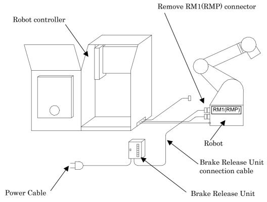
Fig.E.3.1 (b) How to connect brake release unit (In case of except M-410iB)
