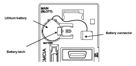
Fig.8.12.1 Replacing the lithium battery
