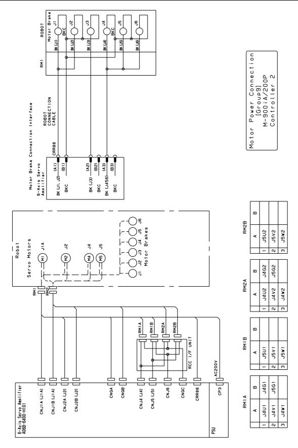
Fig.G.7(p) Motor power connection (Group 9:M-900iA/200P, Controller 2)
