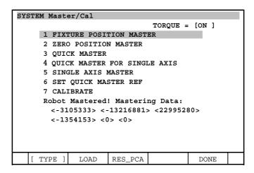
(7) Select "7 CALIBRATE" and press the F4 key (yes). Calibration is performed.
