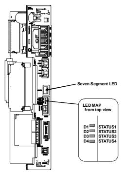
Fig.3.7.1 LED on the main board
