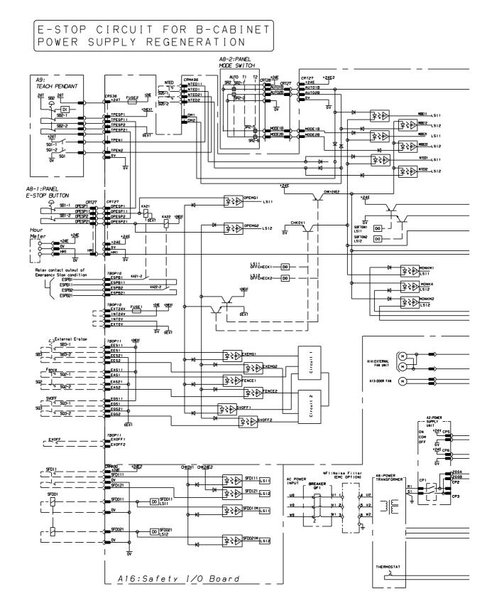
Fig.B (I) Emergency stop circuit connection diagram (B-cabinet/Power supply regeneration)
