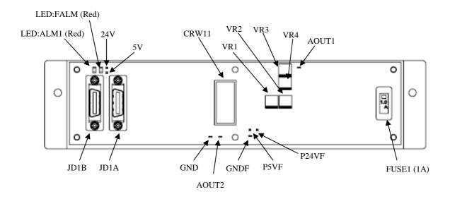
Fig.4.7 Process I/O board MB
