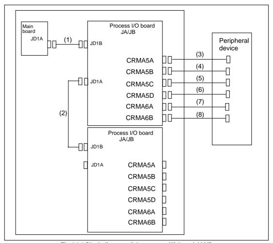
Fig.4.1.1 Block diagram of the process I/O board JA/JB
