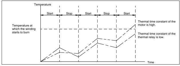
Fig.3.5 (k) Relationship between the temperatures of the motor and thermal relay on start/stop cycles
