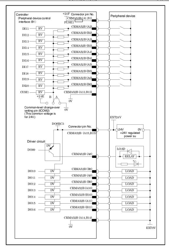
The following shows the connector interface of the optional peripheral device cables on the peripheral device side
