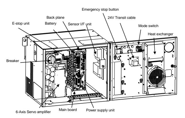
Fig.2.1 (c) R-30iB A-cabinet interior (Front) (CR-35iA)
