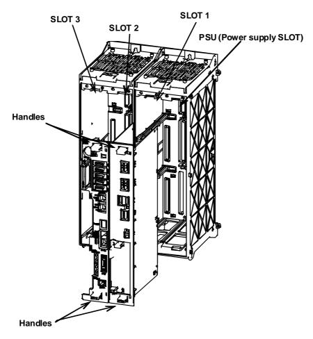
Fig.8.1.2 (b) Replacing the power unit and printed-circuit boards on the backplane
