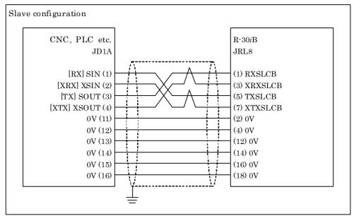
Fig.3.2.2 Connection diagram of I/O Link cable
