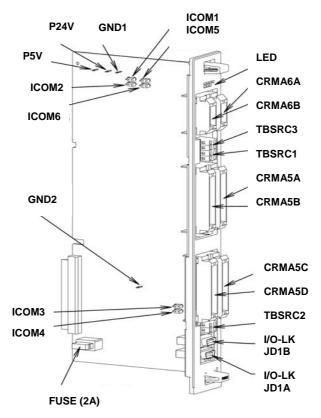
Fig.4.4 Process I/O Board JA
