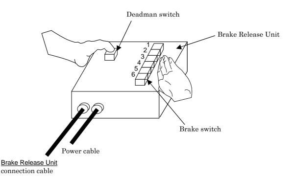
Fig.E.3.1 (a) Brake release unit
