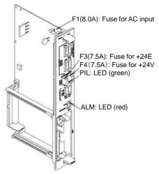
Fig.3.6(a) Fuse on the Power supply unit
