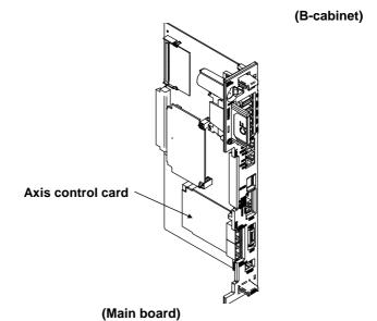
Fig.3.5 (y) SRVO-214 6ch amplifier fuse blown (Panel PCB)
