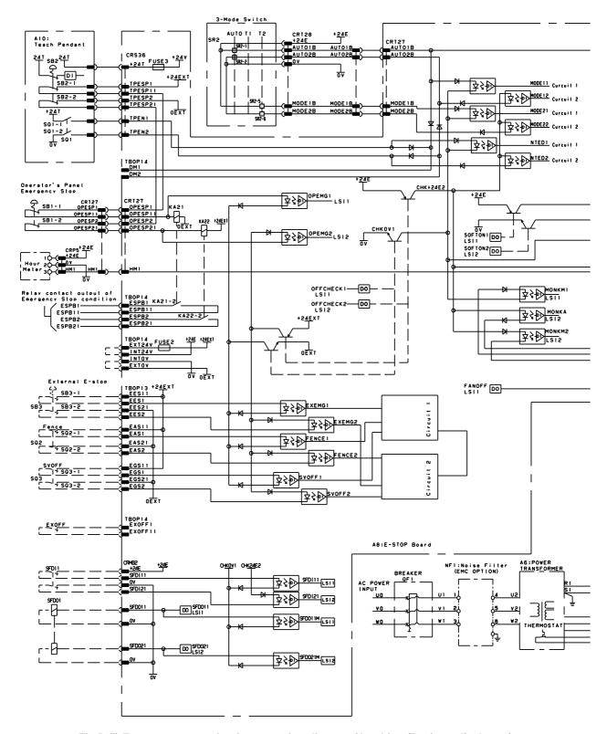
Fig.B (i) Emergency stop circuit connection diagram (A-cabinet/Resistor discharge)
