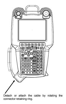
Fig.8.9 Replacing the teach pendant
