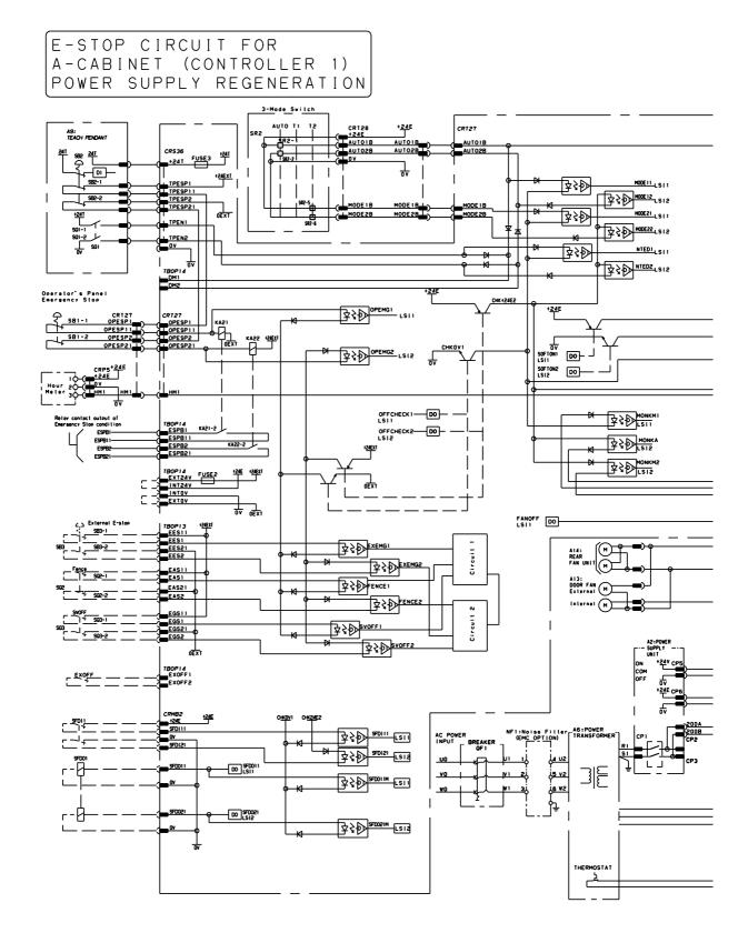
Fig.G.7(g) Emergency circuit connection diagram (A-cabinet/Power supply regeneration/Controller 1)
