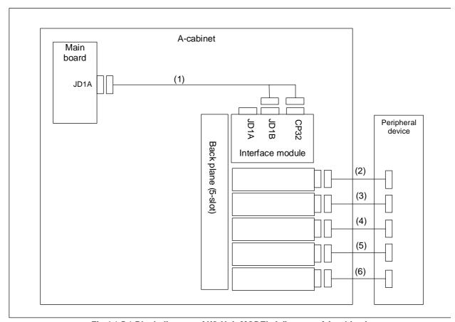
Fig.4.1.5.1 Block diagram of I/O Unit-MODEL A (In case of A-cabinet)
