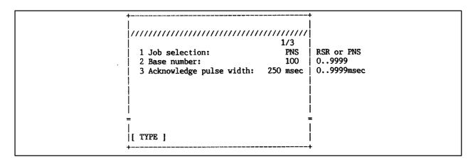
If a number other than zero is entered to PNS input, a program is selected whose program number is the entered value plus the base number. For example, if the PNS value is 23, the program to be started has the program name calculated from the expression
