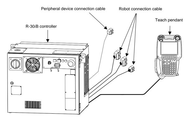
Fig.5.2.2 (a) Assemble at installation (A-cabinet)
