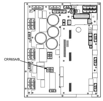
Fig.3.3.7 6-axis servo amplifier
