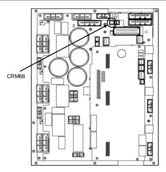
Fig.3.3.8 6-axis servo amplifier
