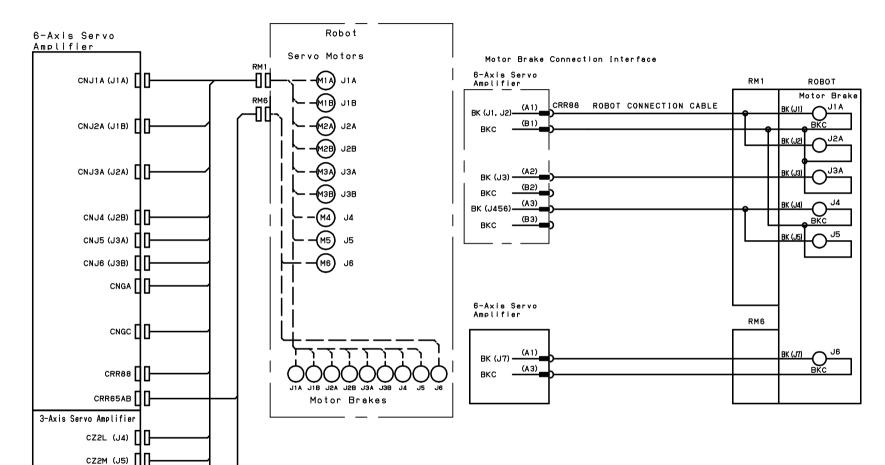
Fig.B (y) Motor Power Connection (group6)
