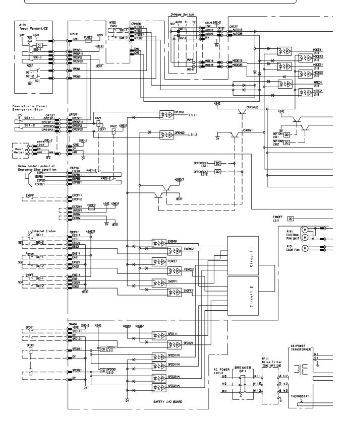
Fig.G.7(i) Emergency circuit connection diagram (B-cabinet/Resistor discharge/Controller 1)
