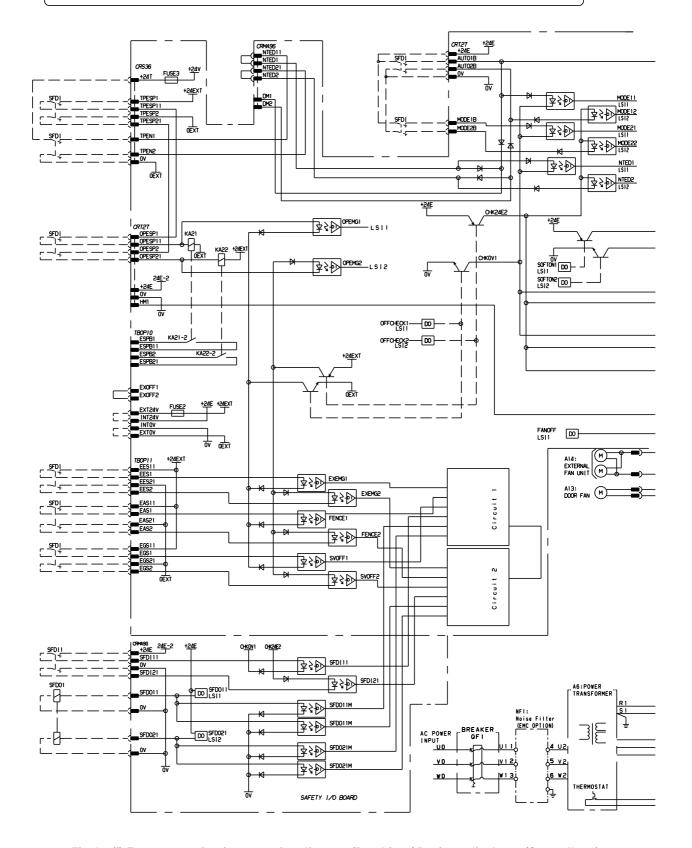
Fig.G.7(j) Emergency circuit connection diagram (B-cabinet/ Resistor discharge/Controller 2)
