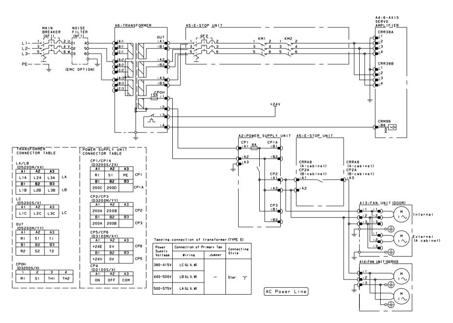
Fig.B (e) AC power line connection diagram Ē case of TYPE Ш transformer)
