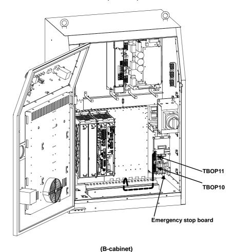
Fig.3.3.5 (a) Connecting the external emergency stop
