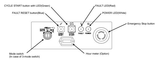
Fig.2.1 (h) R-30iB A-cabinet operator's panel
