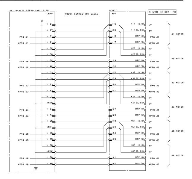
Fig.B (ag) Pulsecoder signal connection diagram (Group1 to 4, 11)
