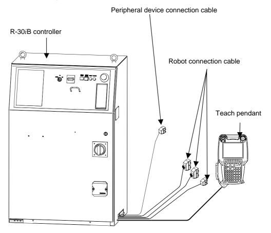
Fig.5.2.2 (b) Assemble at installation (B-cabinet)
