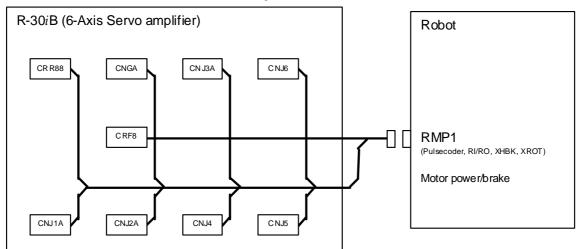
Fig.3.3.1 (g) Robot connection cable (Group8)
