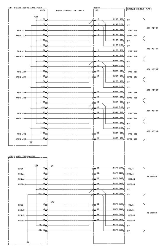
Fig.B (ai) Pulsecoder Signal Connection Diagram (group6; excluding M-430iA/2PH)
