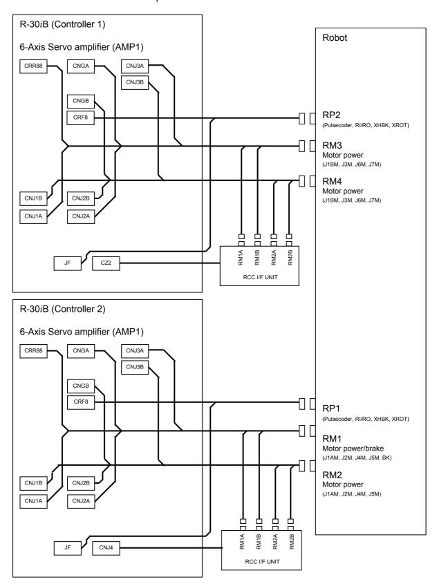
Fig.G.4 (a) Robot connection cable(Group9: M-900iA/200P)
