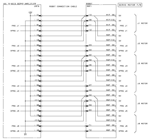
Fig.B (al) Pulsecoder Signal Connection Diagram (Group8; ARC Mate 100iC, ARC Mate 120iC)
