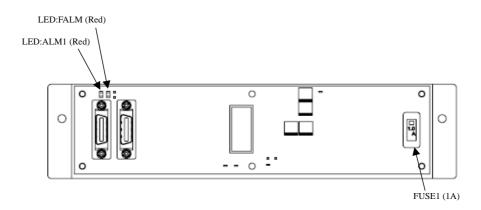
Fig.3.7.4 (c) LEDs on the process I/O board MB
