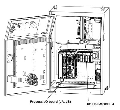
Fig.4(b) Locations of peripheral device interfaces (B-cabinet)
