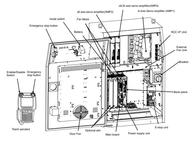
Fig.2.1 (f) R-30iB B-cabinet interior (Front) (M-900 iA/400L, M-900 iA/600, M-900 iB/700, M-900 iB/400L)
