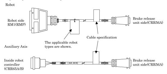
Fig.E.2 Brake release unit connection cable
