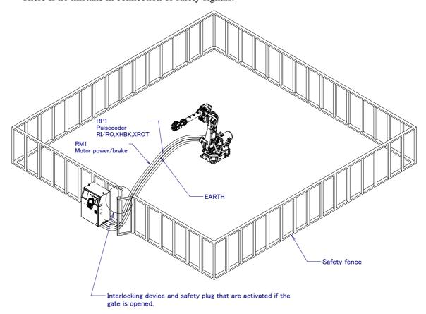
Fig.3 (a) Safety fence and safety gate
