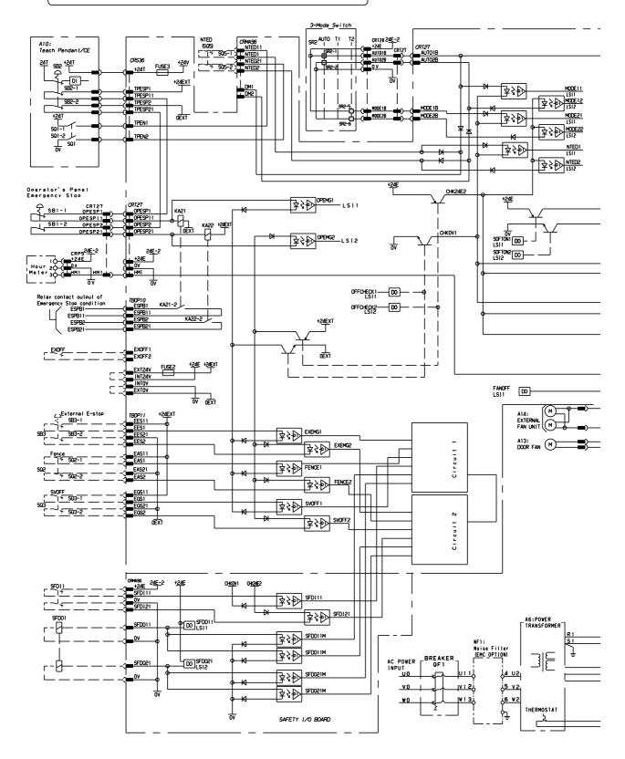
Fig.B (k) Emergency stop circuit connection diagram (B-cabinet/Resistor discharge)
