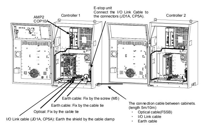
Fig.G.3 Installing the connection cable between cabinets
