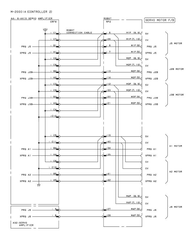
Fig.G.7(x) Pulsecoder signal connection diagram (Group 10:M-2000iA, Controller 2)
