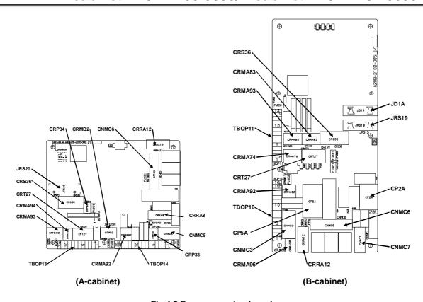
Fig.4.2 Emergency stop board
