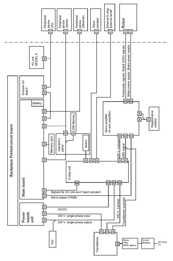
Fig.2.2 Block diagram of the R-30iB
