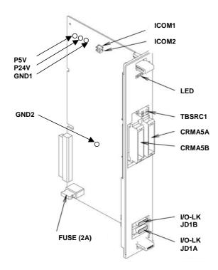
Fig.4.5 Process I/O Board JB
