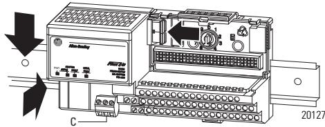
8. If the adapter module does not lock in place, use a screwdriver or similar device to move the locking tab down while pressing the adapter module flush onto the DIN rail, and release the locking tab to lock the adapter module in place. If necessary, push up on the locking tab to lock.
