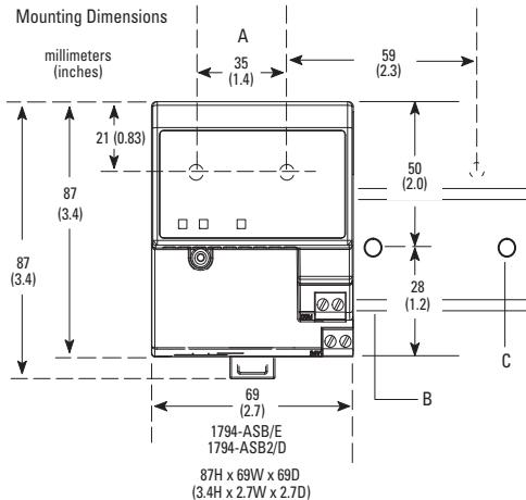
A = Mounting hole dimensions for optional mounting kit
