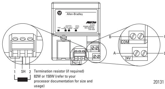
**WARNING** If you connect or disconnect wiring while the field-side power is on, an electrical arc can occur. This could cause an explosion in hazardous location installations. Be sure that power is removed or the area is nonhazardous before proceeding.
